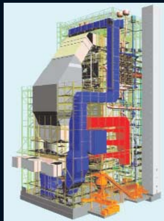
Fig. 3 Walsum #10, supercritical boiler view with dry bottom ash handling system (illustration: courtesy from HPE)
