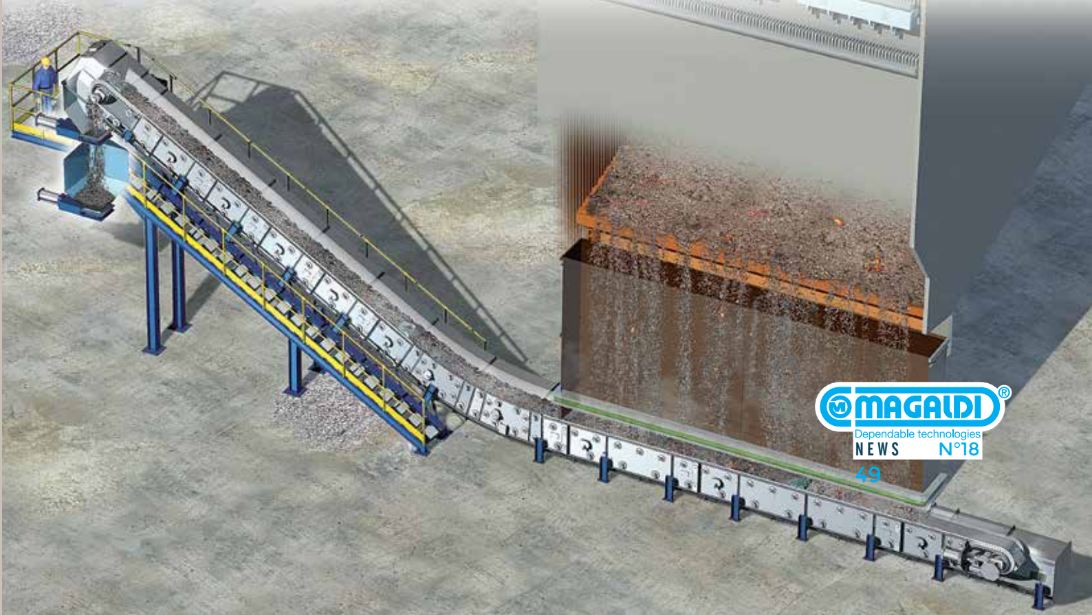
FIGURE 2: POSSIBLE ARRANGEMENT OF THE ECOBELT® BIO.
