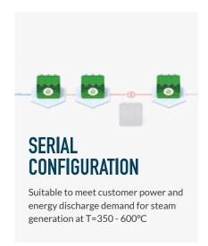
Several modules can be assembled in one MGTES system, in series and/or in parallel to meet the customer power and storage demand, including massive systems with GWh thermal energy storage capacity.
